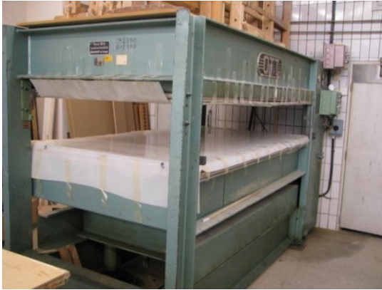
Figure 2.28 Machine to glue the oak
