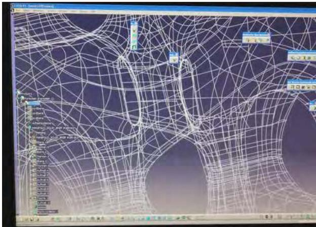
**Figure 2** Screen view of the digital mesh used to mill the shape of a preformed block in Anselm Reyle's aluminum sculpture *Philosophy*, 2009. Used with permission of Anselm Reyle. Photo: Thomas Dempwolf.
