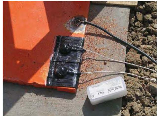
**Figure 11b** The cable connections to the sculpture are coated with a bituminous material to make them waterproof.
