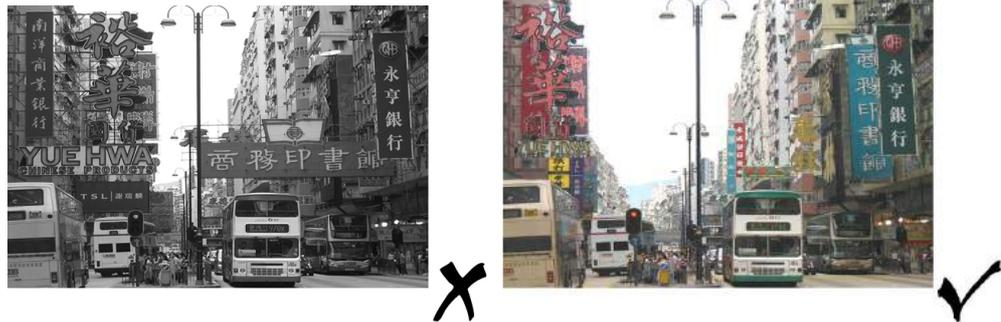
**Figure 54** Projecting Signboards should be Vertical Type instead of Horizontal Type
