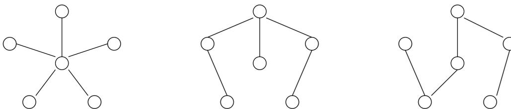
We can immediately notice that their general shape is such that if we add any of the remaining edges, we would create a circle. Then we can see that going from one spanning tree to another can be achieved by removing an edge and replacing it by another (to the vertex which would otherwise be unconnected) such that no circle is created. These observations are not quite sufficient to lead to an algorithm, but they are good enough to let us prove that the algorithms we find do actually work.
