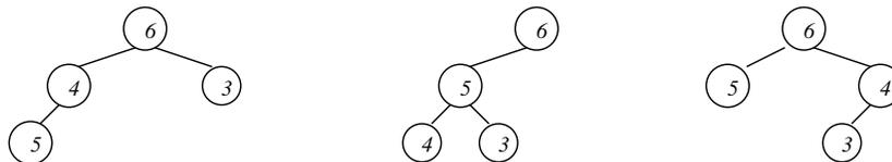
the first because  $5 > 4$  violates the required priority ordering, the second because it is not perfectly balanced and hence not complete, and the third because it is not complete due to the node on the last level not being as far to the left as possible.
