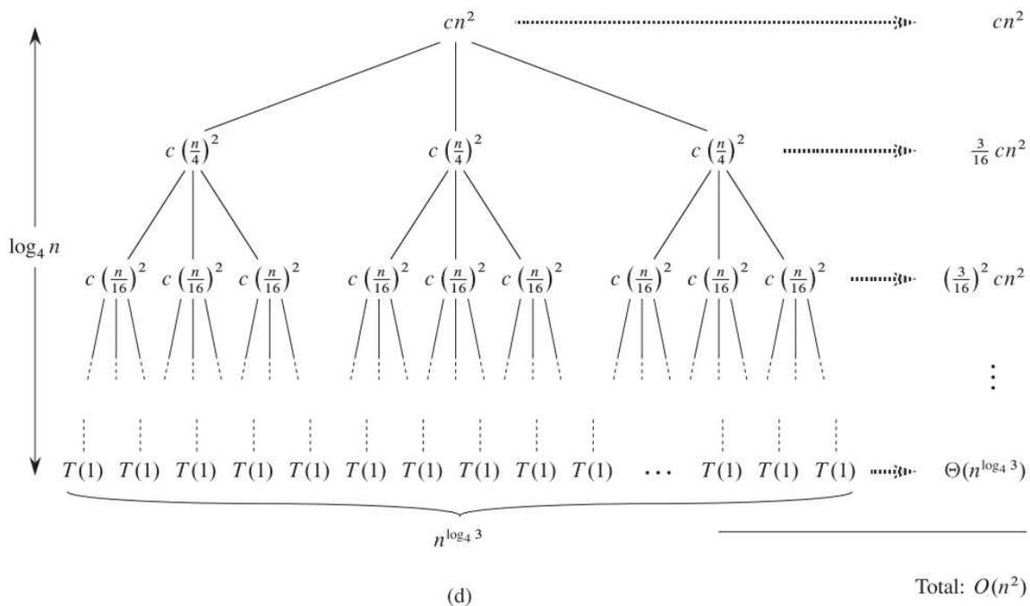
Constructing a recursion tree for the recurrence  $T(n) = 3T(n/4) + cn^2$ . Part (a) shows  $T(n)$ , which progressively expands in (b)–(d) to form the recursion tree. The fully expanded tree in part (d) has height  $\log_4 n$  (it has  $\log_4 n + 1$  levels).
