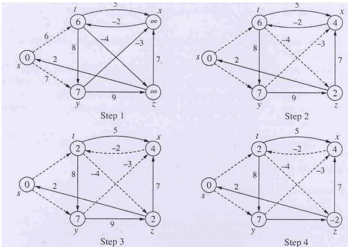
Stepwise working procedure of Bellman Ford Algorithm
