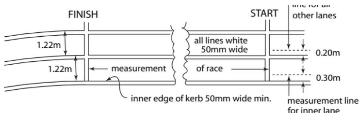
**Figure 160 - Track measurements (infield view)**
