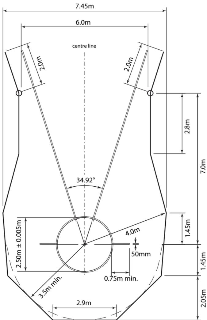
**Figure 192b - Cage for Hammer and Discus Throw with concentric circles
