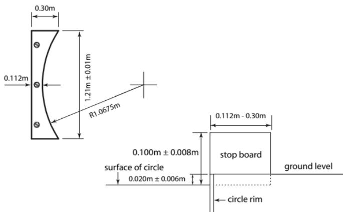
**Figure 188 - Shot Put stop board (top and side view)**
