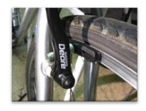
Set the position of the brake pad so that it does not touch the tyre and it does not hangoff the side of the rim when the brakes are applied. Also the pad should meet the rim at 90 degrees.
