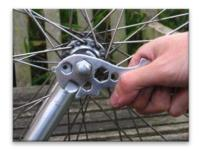
If the puncture is on the front wheel then use the quick release or a wrench to remove the wheel. Turn in an anticlockwise direction to loosen.
