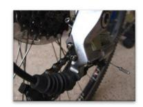
Remember to make adjustments in small quarter turn increments and then re-test by putting the gear cable back into its original position, spin the pedals and change the gears.
