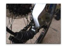
If you notice problems then adjustment is needed. First identify which one is the high and which one is the low screw. These should be marked with a small H and L.
