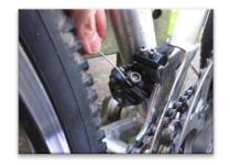
Cable tension is also worth checking. Shift into the largest sprocket in the rear and smallest chainring at the front.
