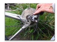
If replacing the rear wheel then push the jockey wheel forward and pull the derailleur backwards. Place the wheel so that the sprockets are within the chain loop. Tighten the bolt or quick release.
