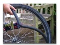
If there is a nut holding the inner tube in position near the valve then undo it. Pull out the inner tube. Then thoroughly inspect the tyre inside and out for anything that may have caused the puncture.
