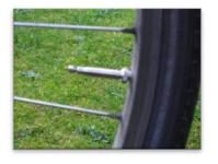
Release any air left inside the tyre by pushing down on the valve head.
