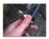
Then turn the chain tool handle until it reaches the chain pin. When it does give it only a 1/3 of a turn.
