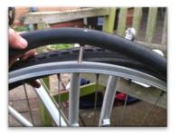
Pump a small amount of air into the inner tube to give it some shape. Then push the valve through the hole. Push the inner tube back inside the tyre.
