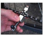
Also work the stiff link in the motion shown above. If this doesn't fix the problem then you will need to use the chain tool. Proceed to the next step.
