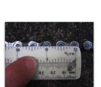
If the pin is less than 1/16<sup>th</sup> of an inch (1.6mm) past the mark then the chain is fine.
