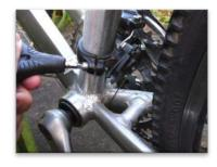
To adjust the derailleur height and angle simply loosen slightly the bolt holding the clamp in place using your Allen key.
