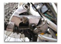
If major adjustment is needed then you may need to loosen the cable fixing bolt to adjust the amount of cable available. If the problem is that the chain is struggling to shift into the next gear then you will need to reduce the amount of slack in the cable.
