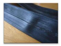
The fun part is finding the puncture. Pump up the inner tube and listen for a hissing sound. Failing that use your lips near the inner tube to feel for any air escaping. You can also try submerging the inner tube in water to watch for escaping bubbles.
