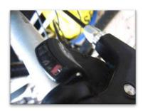
Test out the rest of the gears and make adjustments when problems arise following the steps above to increase or decrease cable tension.
