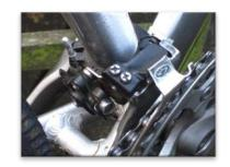
The next adjustment that can be made is to the limit screws. These keep the chain in position so that it does not fall off either side of the chainrings.
