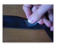
Having found the puncture don't lose it! Use the abrasive paper that came with your puncture repair kit to scrape the area.
