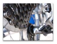
The final adjustment that can be made is to the b-screw. This positions the derailleur angle in comparison to the rear dropout.
