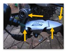
The rear derailleur also needs lubrication to keep working well
