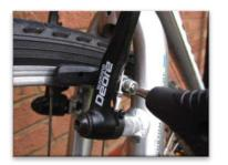
Finally tighten the nut firmly. Tightening the nut can be tricky as when you are tightening it the pad will attempt to move. Try holding it in place with your other hand.
