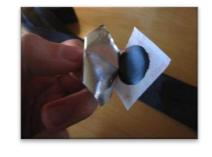
Apply a layer of the glue that comes with the puncture repair kit. You should apply more than what will be needed by the patch and allow it to dry.
