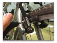
Loosen the bolt holding the brake pad in place then remove it and the washers.
