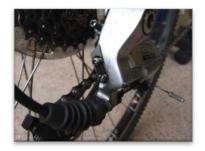
Once you are done with adjustments and have tested you can access all the gears without the chain falling off the edge then work in a tiny bit of lube into the screws.
