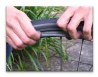
Go to the opposite side of the valve and fold the tyre back over the rim. Work your way around the tyre. This can be a little tough. When you get stuck remove any air from the inner tube. Only if you are really struggling then use the tyre levers to assist.
