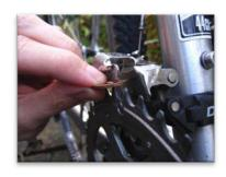
You can use a penny to check to see if there is about 1 to 2 mm of clearance between the outer cage and the highest point of the biggest chainring.
