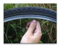
Check the inner tube is underneath the tyre around the whole wheel as if it is caught it will get punctured. Push the valve up into the tyre so that it almost disappears to be sure it is not caught. If there is a nut on the valve screw it back on. Pump up the tyre until it is not possible to push down with your thumb.
