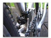
First let's work on the lower limit screw marked L.
