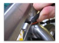
Shift into the largest rear sprocket by pedalling. Then stop pedalling and shift back a couple of gears towards the smaller sprockets. This will give plenty of cable slack so you can pull the gear cable out of its cable stop.
