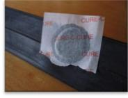
Press the patch down firmly to remove any air.
