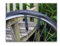
If you don't have tyre levers then work your way around the wheel with your thumbs pushing the tyre off the rim.
