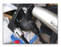
You can make adjustments to the cable tension through the barrel adjuster. This affects how well all the gears perform.
