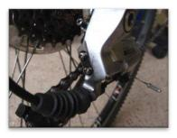
The high and low limit screws stop the chain from falling off the edge of the cassette.
