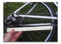
The easiest way to measure for chain wear is to measure the length of 12 links. These should measure 12 inches.
