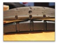
Check the brake pad surface. As you can see the top one is completely worn out. In the worn out one the grooves have completely disappeared.
