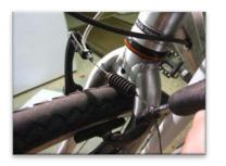
If more adjustment is needed than the barrel adjuster can provide then loosen the cable clamp bolt. Then either release cable or pull more cable in. Finally retighten the bolt and test the wheels spin without touching the pad.
