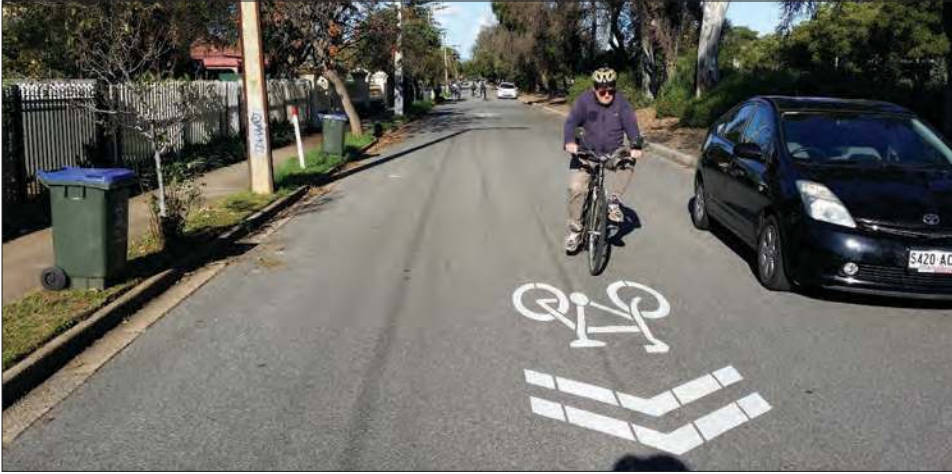
Figure 12.7: A neighbourhood greenway in Adelaide, South Australia, featuring 'sharrow' markings. (Source: Author.)
