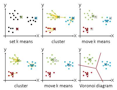
The algorithm has converged when the assignments no longer change. It is often presented as assigning objects to the nearest cluster by distance.
