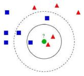
The test sample (green dot) should be classified either to blue squares or to red triangles.
