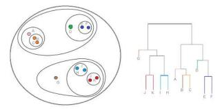
The advantage of Hierarchical Clustering is we don't have to pre-specify the clusters. However, it doesn't work very well on vast amounts of data or huge datasets. And there are some disadvantages of the Hierarchical Clustering algorithm that it is not suitable for large datasets.
