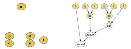
The example shows how six different clusters (data points) are merged step by step on distance until they all create one large cluster.
