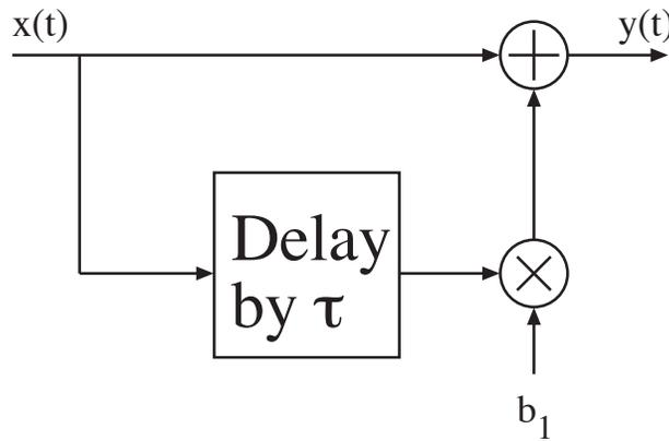
Figure 3.5: A basic feedforward filter block diagram.
