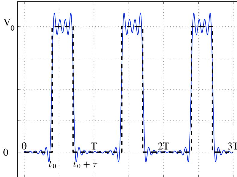
Figure 1.10: The Fourier series for a periodic sequence of rectangular pulses. The first 12 harmonic terms in summation (1-62) are included. The ideal pulse train is shown as dashed lines. The period is  $T = 1$ , the initial point  $t_0 = 0.5$  and the pulse width  $\tau = 0.3333$ .
