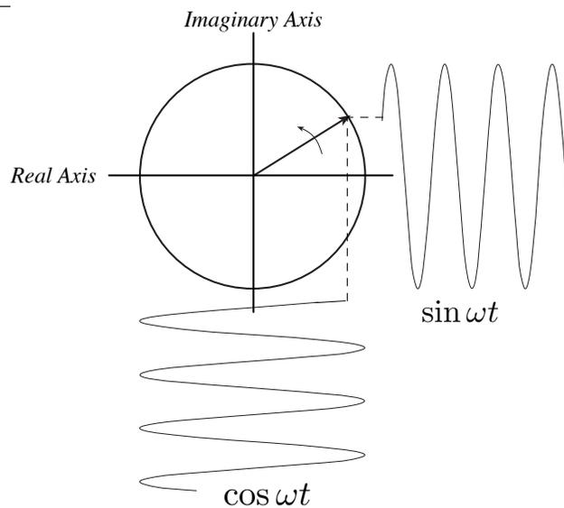
Figure 1.4: Components of a phasor are sinusoids.
