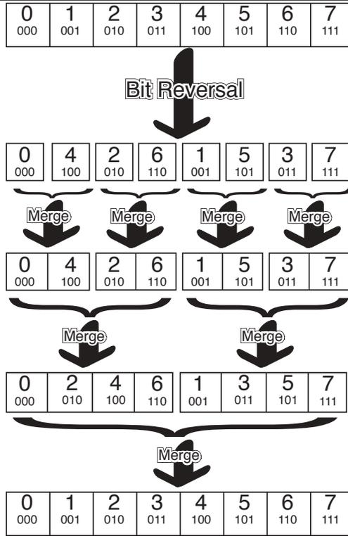
Figure 6.6: Schematic outline of an iterative 8-point FFT
