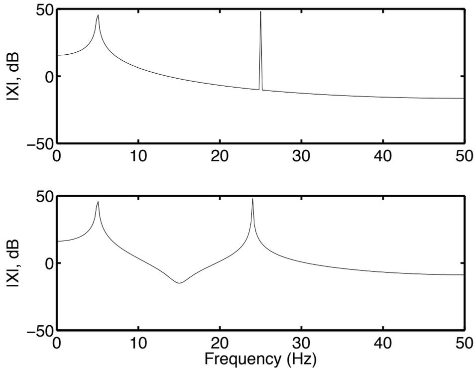
Figure 6.8: Similar input signals as in figure 6.7, but here the two frequencies are  $f_1 = 5\text{Hz}$  and  $f_2 = 25\text{Hz}$  for the top plot and  $f_1 = 5\text{Hz}$  and  $f_2 = 24\text{Hz}$  for the bottom.
