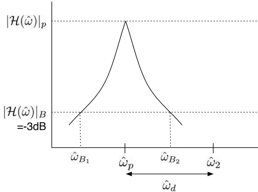
Figure 5.6: Designing a simple one-pole feedback filter. A filter’s frequency response is sketched for the situation where we want the center of its passband at  $\hat{\omega}_p$  and we wish to ensure that another frequency,  $\hat{\omega}_2 = \hat{\omega}_p + \hat{\omega}_d$ , is well outside the passband. We choose the filter’s cutoff frequencies,  $\hat{\omega}_{B1} = \hat{\omega}_p - \hat{\omega}_B$  and  $\hat{\omega}_{B2} = \hat{\omega}_p + \hat{\omega}_B$ , to achieve this.
