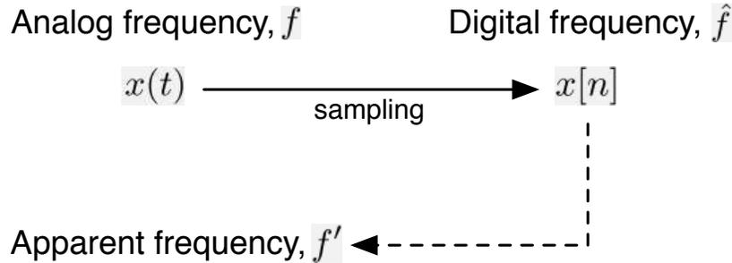
Figure 2.3: Sampling an analog signal,  $x(t)$ , with an analog (actual) frequency  $f$  produces a digital signal,  $x[n]$ , at a digital frequency  $\hat{f}$ . If one examines that digital signal and converts  $\hat{f}$  back to an analog frequency, the apparent frequency is  $f'$ , which may not be the same as  $f$ , due to aliasing.
