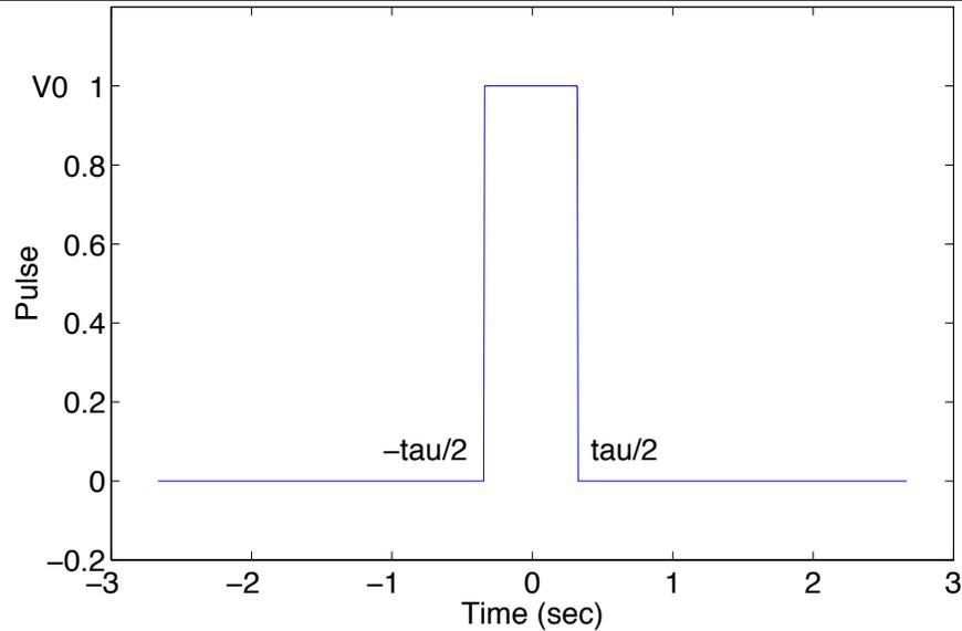
Figure 6.1: A rectangular pulse with width  $\tau$ .
