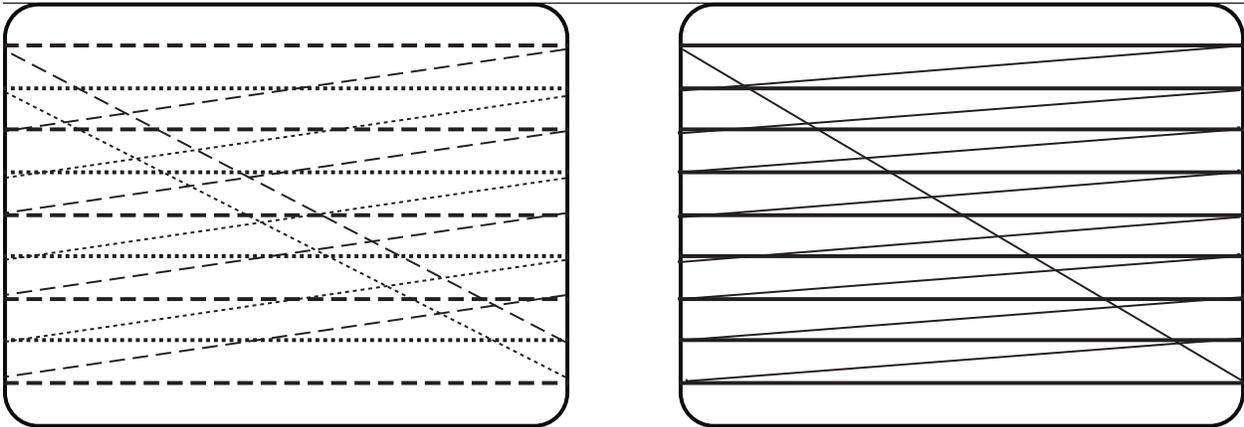
Figure 1.2: Interlaced (left) and non-interlaced (right) raster scanning.
