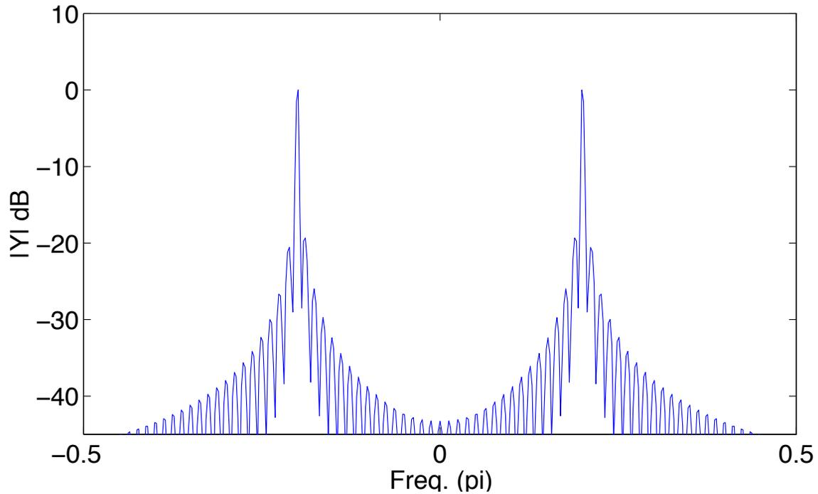
Figure 6.9: Magnitude spectrum of windowed signal  $x[n] = \cos \hat{\omega}_0 n$ ,  $\hat{\omega}_0 = 0.2\pi$  and the rectangular window length is  $N = 128$ . This illustrates the occurrence of power leakage.
