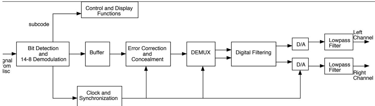
Figure 9.2: Simplified block diagram of a CD player.
