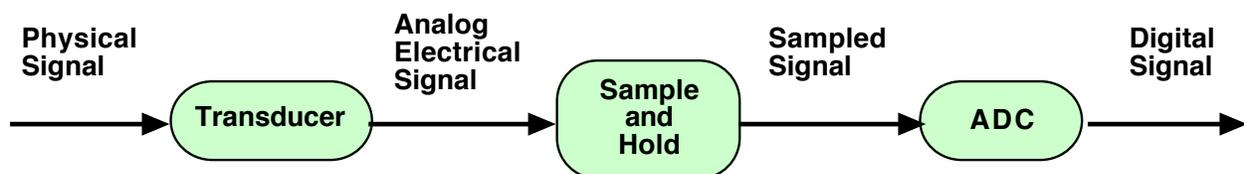
Figure 2.1: Block diagram of the data acquisition process.
