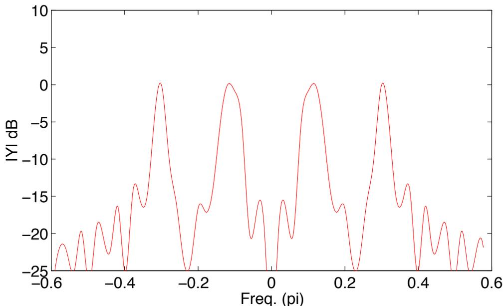
Figure 6.11: Magnitude spectrum of the signal (6-55) made up of three sinusoids.  $\hat{\omega}_0 = 0.1\pi$ ,  $\hat{\omega}_1 = 0.12\pi$ ,  $\hat{\omega}_2 = 0.3\pi$ , and the rectangular window length was  $N = 16$ . Because of the small window size,  $\hat{\omega}_0$  and  $\hat{\omega}_1$  are indistinguishable.
