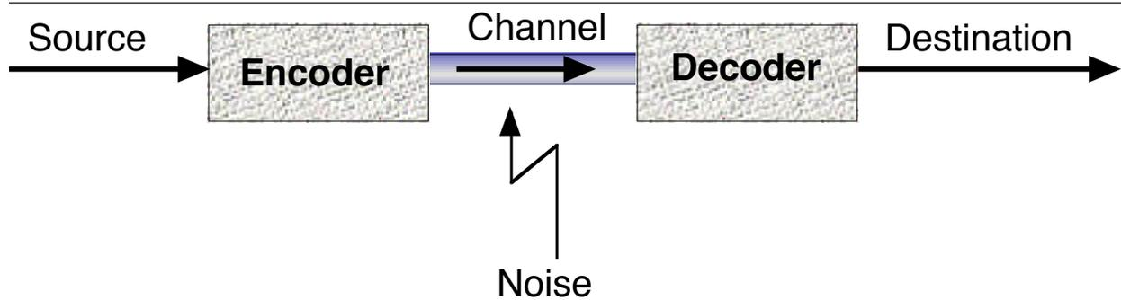
Figure 7.1: Shannon's model for coding information for transmission.
