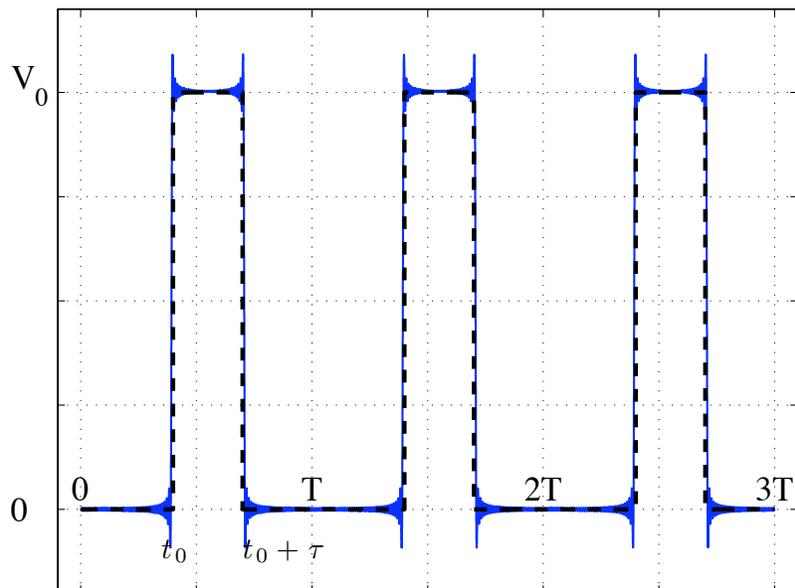
Figure 1.11: The Fourier series for a periodic sequence of rectangular pulses. The sum of the first 100 terms is shown, as in figure 1.10.
