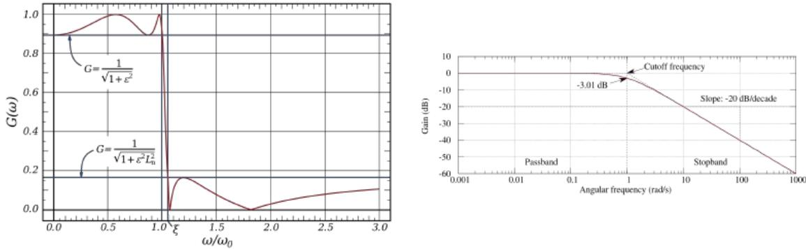
Figure 5.7: Example filter frequency responses: elliptic (left)<sup>1</sup> and Butterworth (right)<sup>2</sup>.
