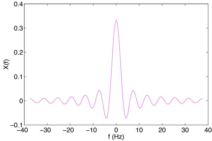
Figure 6.2: Fourier transform of the pulse in figure 6.1.
