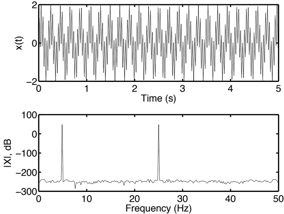
Figure 6.7: Sum of two sinusoids  $x$  with  $N = 512$  samples (top) and its FFT  $|X|$  (bottom). The sampling frequency is  $f_s = 100\text{Hz}$ ,  $f_1 = 25\Delta f = 4.8828\text{Hz}$  and  $f_2 = 128\Delta f = 25.0\text{Hz}$ , where frequency step  $\Delta f = f_s/N = 0.1953\text{Hz/sample}$ .
