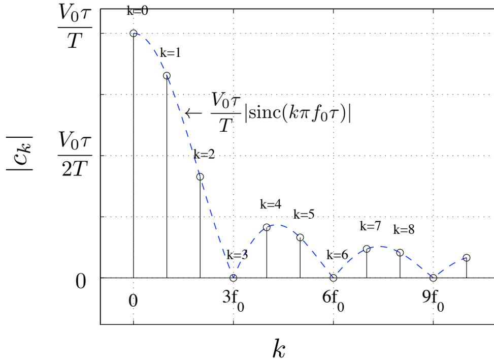
Figure 1.12: The spectrum of a periodic sequence of rectangular pulses: the magnitude of  $c_k$  vs. frequency  $f = kf_0$ , where  $f_0 = 1/T$  (light gray vertical lines). The envelope for continuous  $k$  is plotted as the black curve. Zero points in the spectrum  $|c_k|$  are at  $kf_0 = n/T = m/\tau$ ,  $m = 1, 2, 3, \dots$
