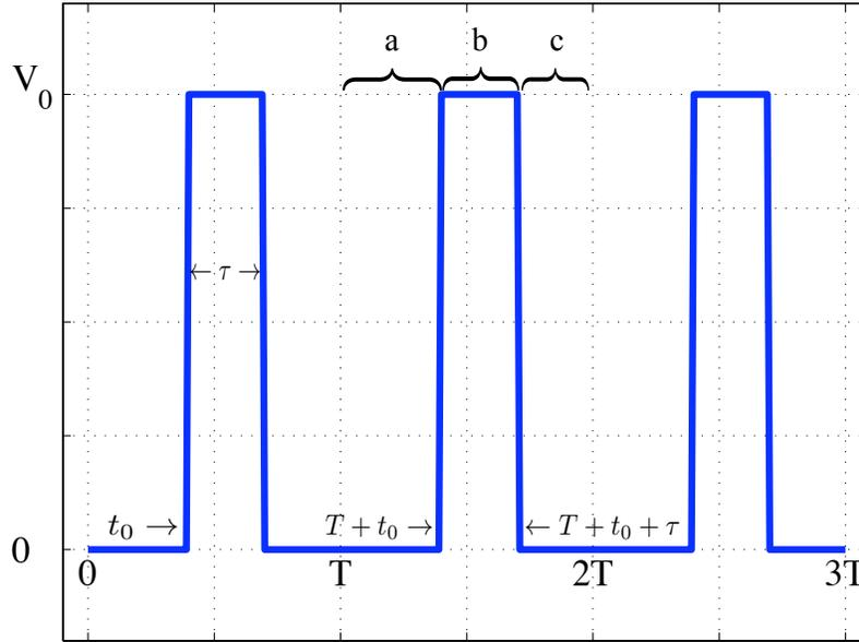
Figure 1.8: A train of periodic rectangular pulses with period  $T$ , pulse width  $\tau$ , and initial pulse start at  $t_0$ .
