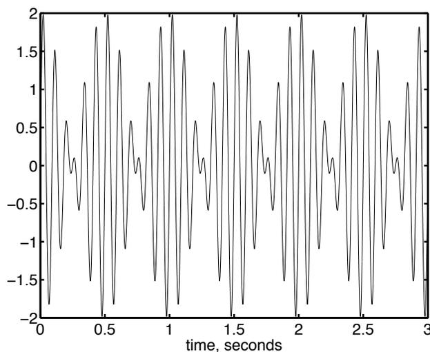
Figure 1.7: Amplitude vs. time representation of beating.
