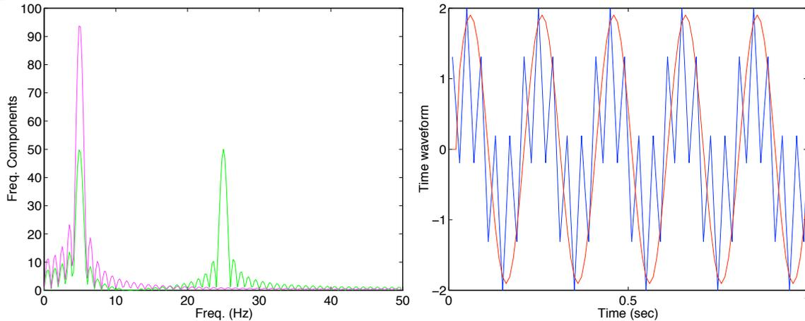
Figure 3.10: The spectrum of a two frequency component sine wave and its filtered version, using the feedforward filter  $y[n] = x[n] + x[n - 2]$ ,  $f_1 = 5Hz$  and  $f_2 = 25Hz$ . Zeros are at  $z_0 = 0.99e^{\pm j\pi/2}$ . The time waveforms are also shown.
