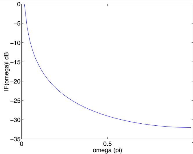
Figure 4.3: Frequency content of the unit step signal.
