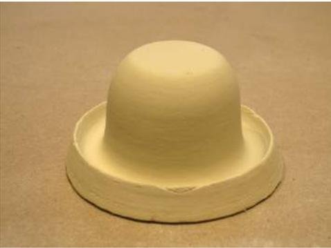
Figure 7: Glaze Bell for potentially runny glazes. From Mark Palandri's Blog at palandri.com
