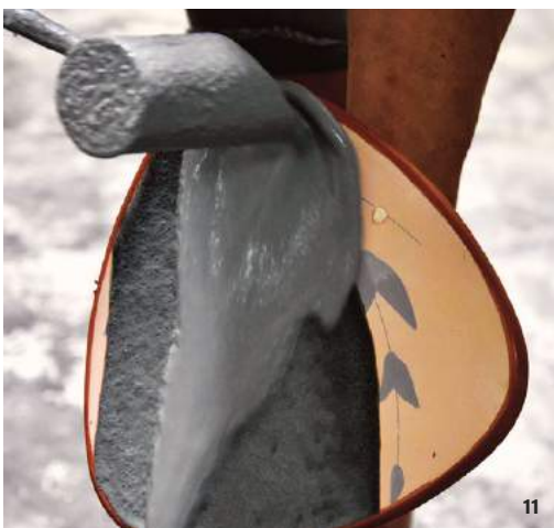
Pour an ash glaze over the face of the plate using a ladle.
