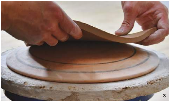
Transfer the slab to a hump mold, making sure the shape is centered on the mold.
