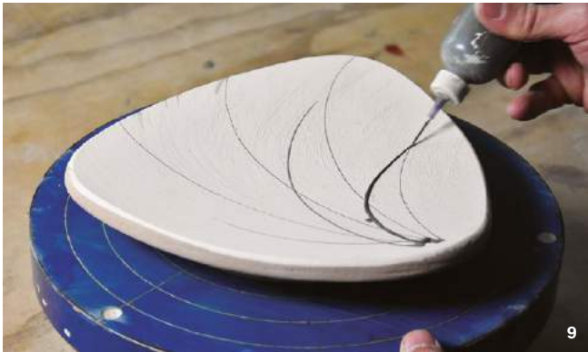
Starting in one corner, slip trail the stems of the grass pattern in a fan shape across the plate.
